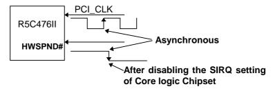
12. PCI signals of other PCI devices should not keep active when VCC\_PCI of R5C476II is turned off in hardware suspend mode.
