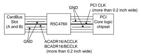
6. Apply wide-width (more than 0.2 inch (0.5mm)) traces and wire as short as possible for these signals below.
