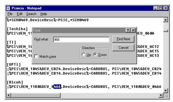
6) Remove the semi-colon in front. Change the strings from "0466" to "0476" as shown below. [Ricoh]
