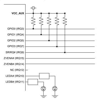
19. In the Serialized IRQ mode, please design that the fall of the SRIRQ# will have **more than 5ns Hold time** for the raise of PCI\_CLK which is input to the R5C476II.
